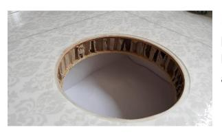
Lightweight panels are usually panels reinforced with cardboard honeycomb, e.g. IKEA construction are not suitable for installation
